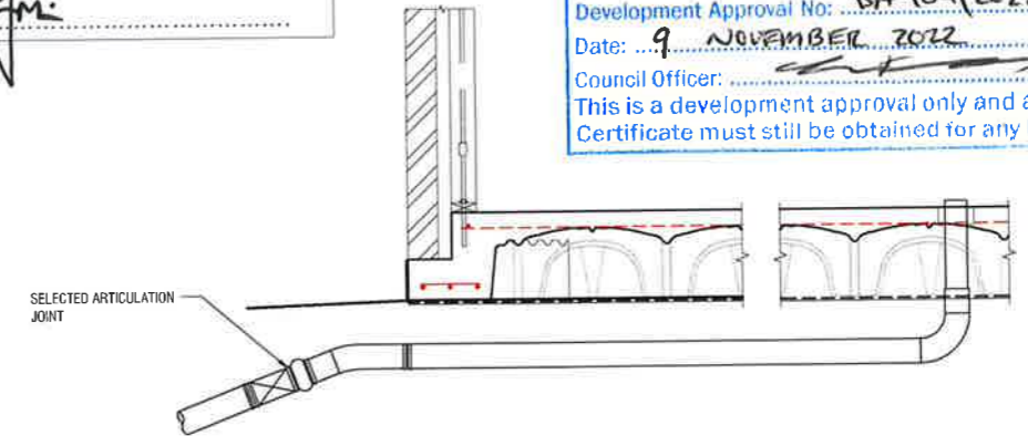
TYPICAL SERVICE PENETRATION THROUGH SLAB N.T.S.
