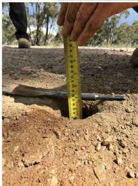
TP 11 - Waterloo Road The material encountered was brown coloured sandy gravel road base material with the majority of the material a minus 40mm which was down to a depth of 70mm
