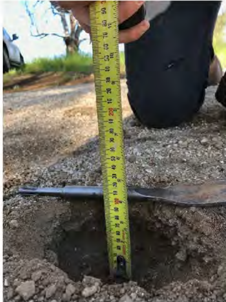
TP 14 – Western Feeder Road The material encountered was brown coloured sandy gravel road base material with the majority of the material a minus 40mm which was down to a depth of 100mm
