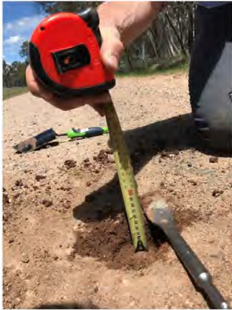
TP 1 – Waterloo Road The material encountered was brown coloured sandy gravel road base material with the majority of the material a minus 40mm which was down to a depth of 50mm
