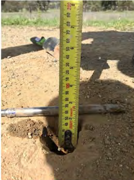
TP 10 - Waterloo Road The material encountered was brown coloured sandy gravel road base material with the majority of the material a minus 40mm which was down to a depth of 50mm
