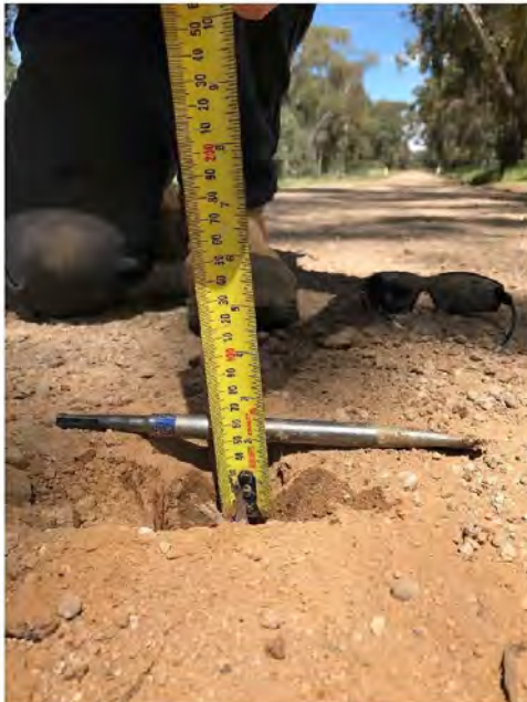
TP 7 - Waterloo Road The material encountered was brown coloured sandy gravel road base material with the majority of the material a minus 40mm which was down to a depth of 50mm
