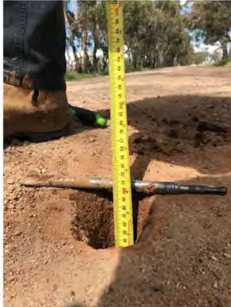
TP 8 - Waterloo Road The material encountered was brown coloured sandy gravel road base material with the majority of the material a minus 40mm which was down to a depth of 100mm
