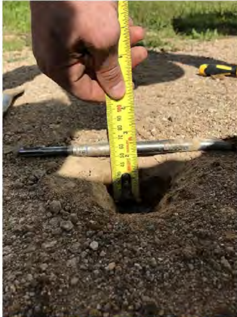
TP 12 – Western Feeder Road The material encountered was brown coloured sandy gravel road base material with the majority of the material a minus 40mm which was down to a depth of 50mm
