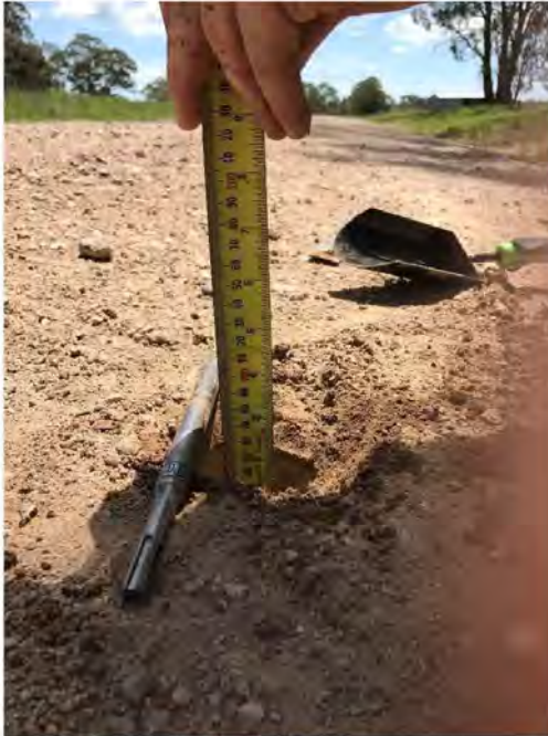
TP 2 – Waterloo Road The material encountered was brown coloured sandy gravel road base material with the majority of the material a minus 40mm which was down to a depth of 60mm
