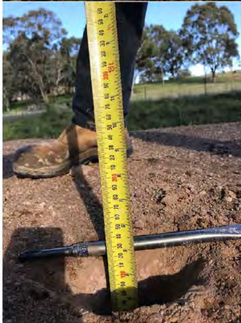
TP 13 – Western Feeder Road The material encountered was brown coloured sandy gravel road base material with the majority of the material a minus 40mm which was down to a depth of 120mm
