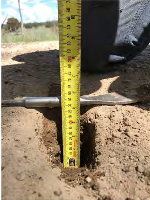
TP 6 - Waterloo Road The material encountered was brown coloured sandy gravel road base material with the majority of the material a minus 40mm which was down to a depth of 120mm
