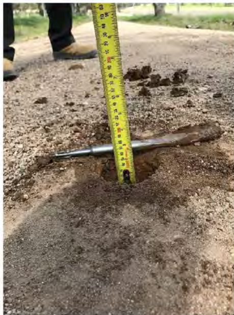
TP 9 - Waterloo Road The material encountered was brown coloured sandy gravel road base material with the majority of the material a minus 40mm which was down to a depth of 60mm
