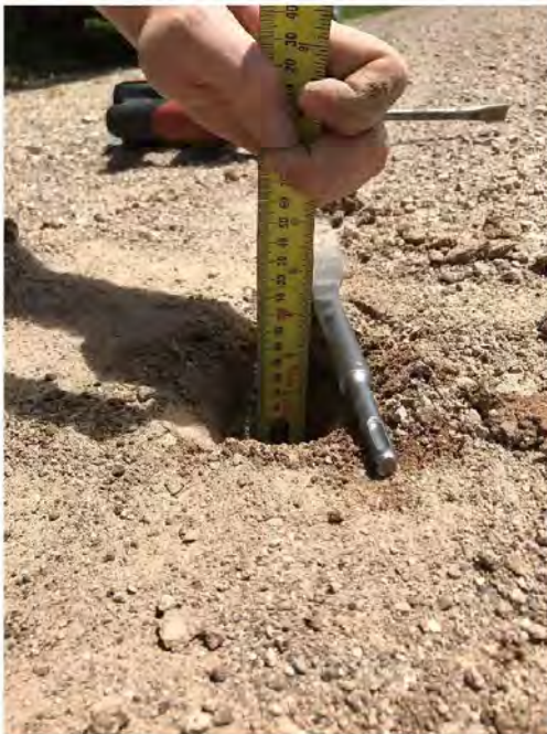
TP 3 – Waterloo Road The material encountered was brown coloured sandy gravel road base material with the majority of the material a minus 40mm which was down to a depth of 60mm
