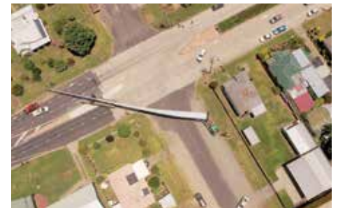
Wind turbine blade navigating the turn from New England Highway to Heron Street in Glen Innes.
